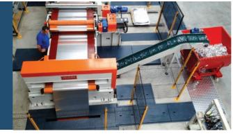
Standard and High-Precision Trimming Shears with automatic positioning of the cutting heads and high-speed operation on thicknesses 0,10 ÷ 5 mm. The accuracy of the radial and axial rotation of the heads ensures very high cutting accuracy and virtually no burrs.
