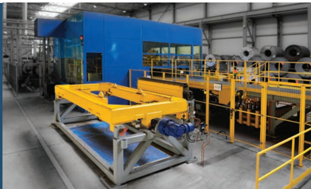
Large Cassette Overturning Device for Heavy Gauge Levelers
